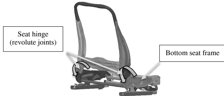
Figure 3. Toyota Yaris FE seat model (seat frame)
