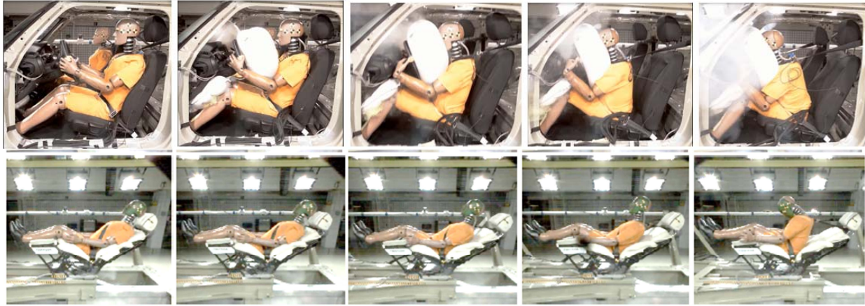
Figure 1: Dummy kinematics comparison: conventional seating configuration, above, and the prototype reclined configuration below, from [4].
